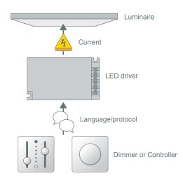
DT8 is the 'color-aware' control standard for all Tunable White applications LED driver technology based on color science enables end-to-end solutions Broad product offering for downlight, track and linear applications, constant voltage and constant current, from 10W to 100W.
